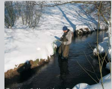
Measuring vertical temperature profiles to invert exchange rates at the River Eger, Photo: J. Fleckenstein, UBT
